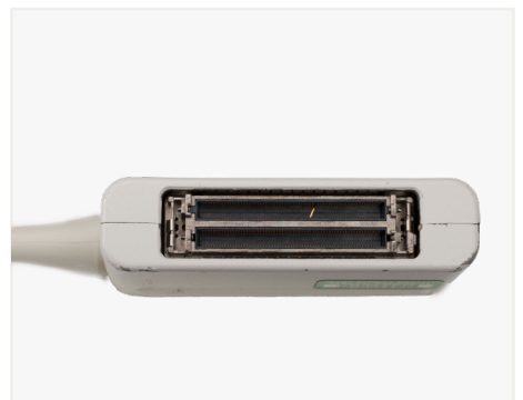
Bent/Damaged Connector Pins
