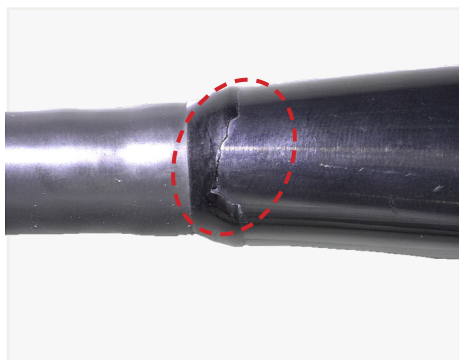
Damaged Glue Bead
