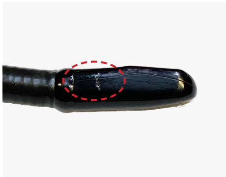
Cracked Distal Tip
