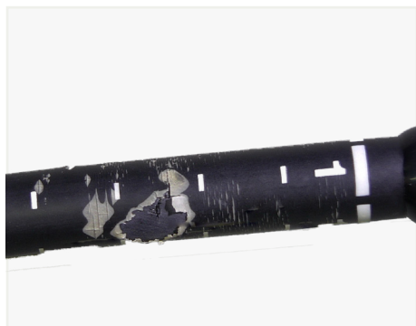
Cut/Damaged Insertion Tube
