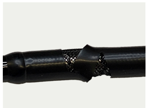
Cut/Damaged Bending Rubber
