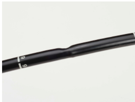
Crushed/Dented Insertion Tube
