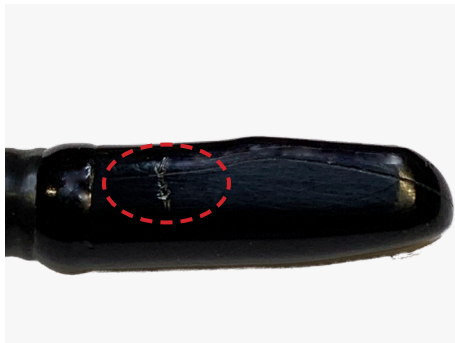
Cracked Distal Tip
