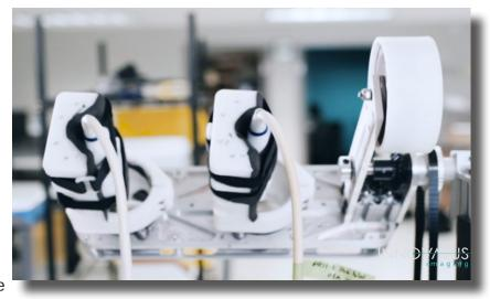
much of the flexing occurs. The Cable Flex Test continuously twists and flexes the cables and strain reliefs of new and repaired probes to determine the point that performance is diminished.
