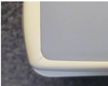
Cracked Probe Housing
