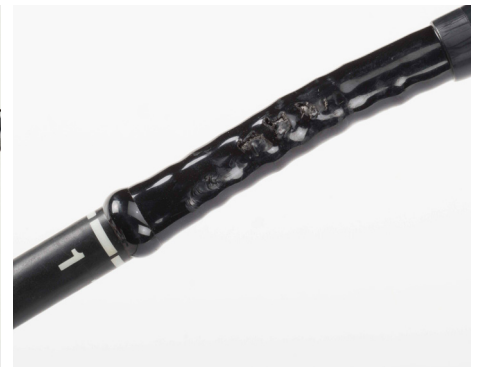
Cut/Damaged Bending Rubber
